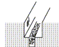
Close-up of crack Before filling
